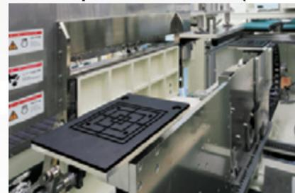
Transport adsorption table is exchangeable.
