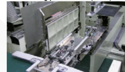
Panel support can prevent the bending for the thin panel.
